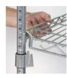
The tubular posts with rolled circular grooves at 1 inch increments are clearly numbered to make assembly exceptionally easy, fast, and accurate. No tools are required for assembly or adjustment. The built in tapered corner shelf collar mates perfectly with the interlocking clip. Mating rib ensures positive shelf positioning.
